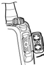
2. Align the accessory (such as an audio accessory or a programming cable) plug with the accessory connector.
