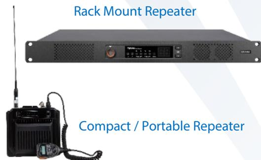
The repeater typically consists of a receiver, transmitter, and a duplexer. The receiver receives incoming radio signals and filters them to ensure that only the desired signals are transmitted to the transmitter. The transmitter then amplifies and retransmits the signal over a wider area. The duplexer is used to separate the incoming and outgoing signals, allowing the repeater to operate on two frequencies (Tx and Rx) on one antenna.
