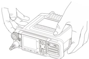
2. Hold the front panel, and then pull and remove the plastic upper cover.
