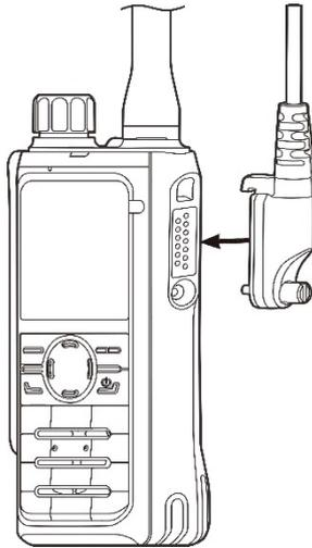
3. Tighten the screw on the audio accessory plug.
