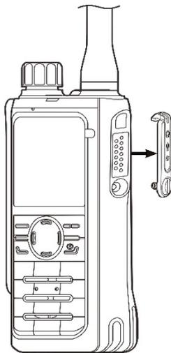
2. Insert the audio accessory plug into the accessory connector.
