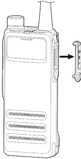
2. Insert the audio accessory plug into the accessory connector.
