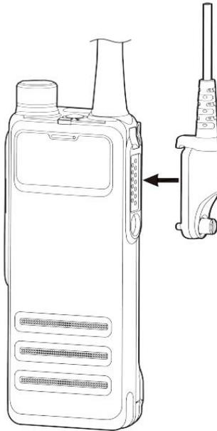
3. Tighten the screw on the audio accessory plug.
