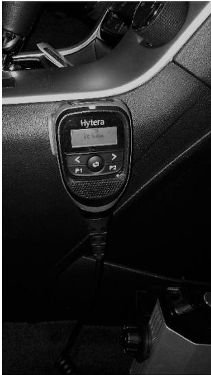
Mount the mic clip on a solid, steady surface that is easily accessible for the user
