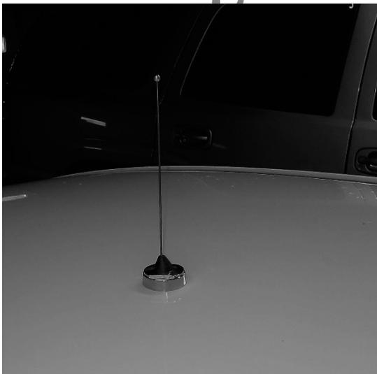
Attach antenna to the roof mount and snug with a crescent wrench
